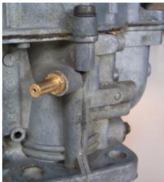
*4-mm hole, and cutting M5-thread into the dual choke carburettor (see photo) because these are already prepared for a vacuum nipple. The nipple is supplied with the 123\EVO.*
